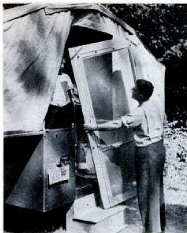
Above, screen-door unit bolts to door opening and tent flaps button to doorframe. Right, screen-door unit stores in well under trap door in trailer floor
